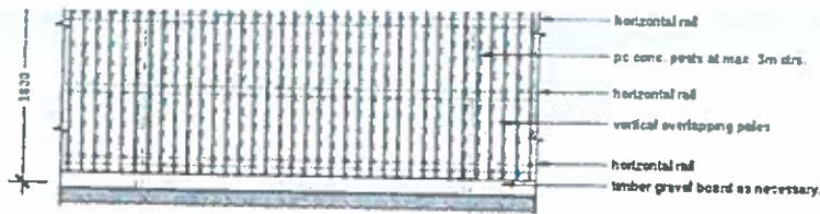
TYPICAL CLOSE BOARDED TIMBER FENCE DETAIL (1:50)
